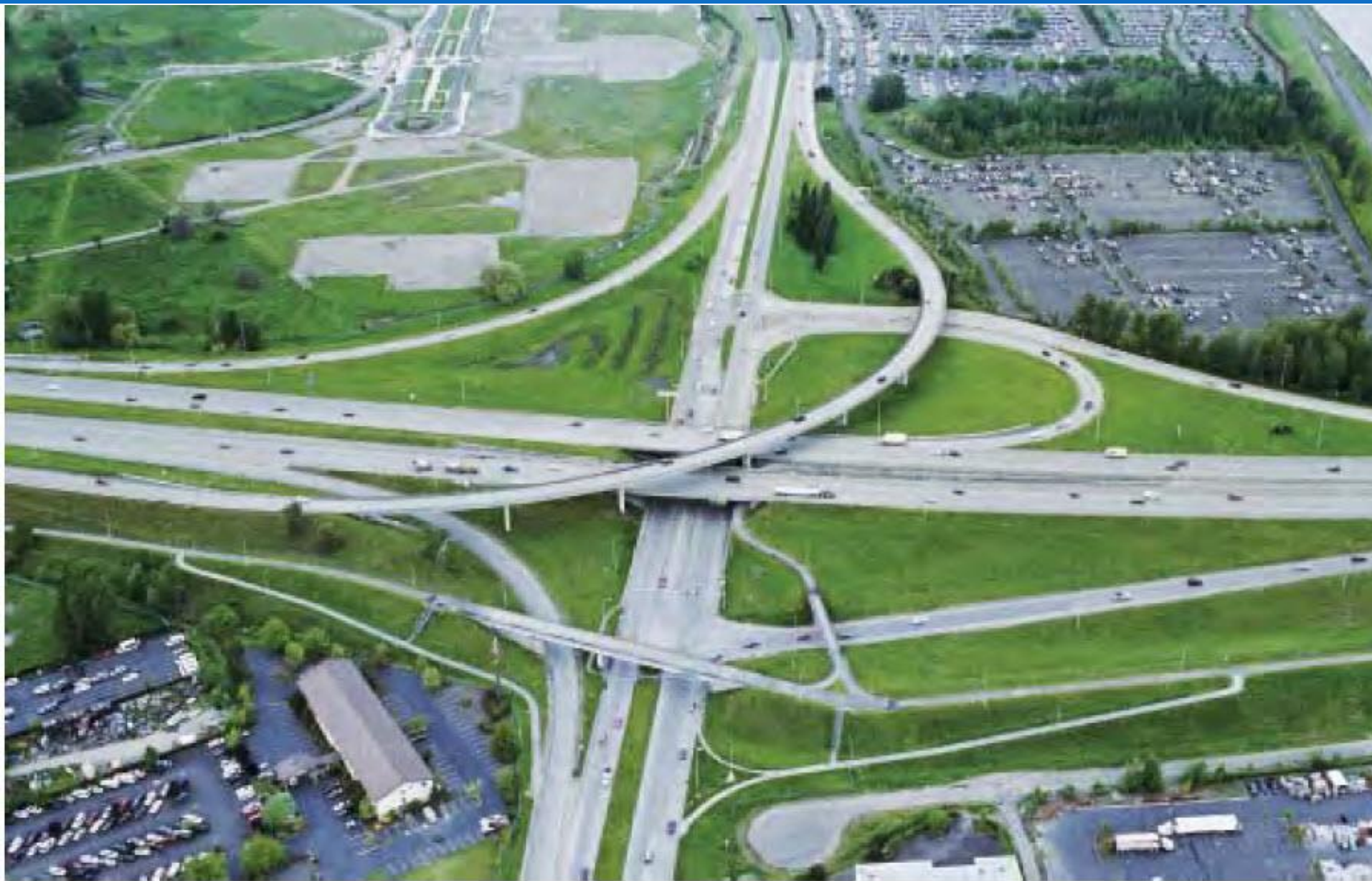
Figure 10-40. Four-Leg Interchange, Diamond with a Direct Connection
