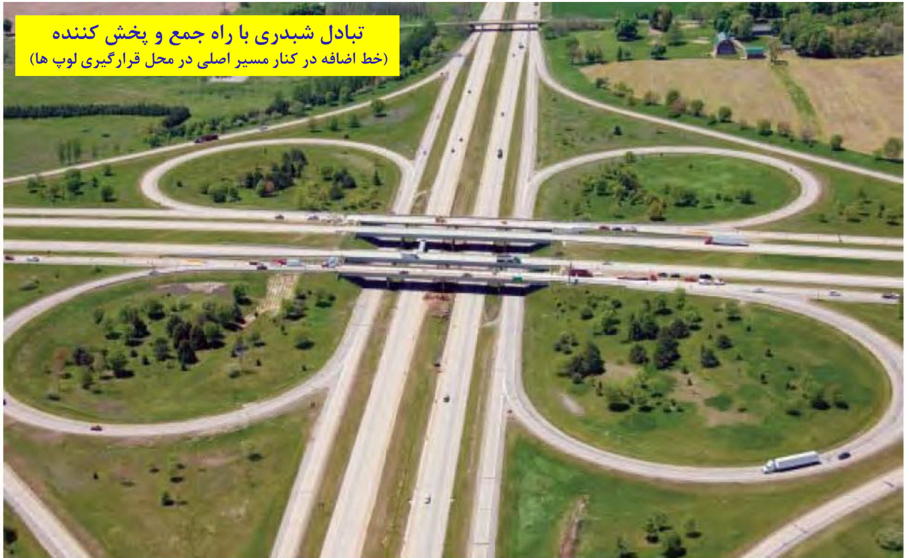
Figure 10-28. Four-Leg Interchange, Cloverleaf with Collector-Distributor Roads
